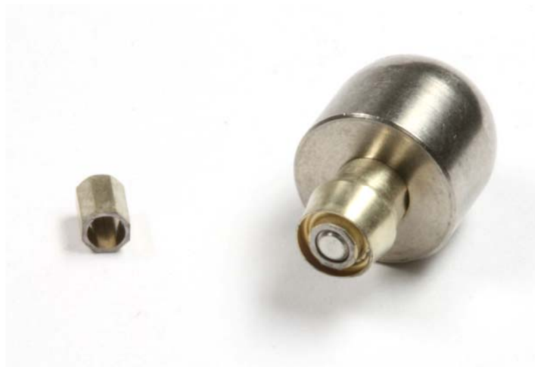
Fig. 5: Fracture of the prosthetic screw after the dynamic test – specimen 1.6.
